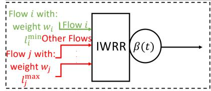
If the strict service curve of the aggregate is a rate-latency (  $\beta(t)=\beta_{c,T}$ ), then  $\beta_{r_0^*,T_0^*}(\beta(t))$  and  $\beta_{r_{\nu^*},T_{\nu^*}^*}(\beta(t))$  are also rate-latency.
