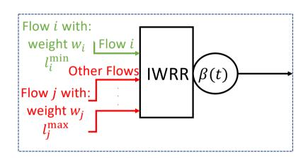
$$\beta(t-s) \leq (R_i^*(t) - R_i^*(s)) + \sum_{j,j \neq i} R_j^*(t) - R_j^*(s) \quad \text{($\beta$ is the strict service curve of server)}$$
